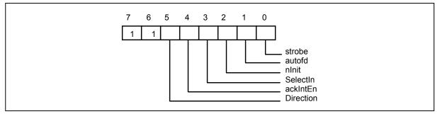
Bit 6, 7: These two bits are logic one during a read and cannot be written.
