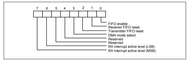
Bit 6, 7: These two bits are used to set the active level for the receiver FIFO interrupt. For example, if the interrupt active level is set as 4 bytes, once there are more than 4 data characters in the receiver FIFO, the interrupt will be activated to notify the CPU to read the data from the FIFO.
