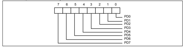
The contents of DB0-DB7 are buffered (non-inverting) and output to ports PD0-PD7 during a write operation. The leading edge of  $\overline{IOW}$  causes an EPP address write cycle to be performed, and the trailing edge of  $\overline{IOW}$  latches the data for the duration of the EPP write cycle.
