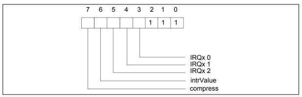
Bit 7: This bit is read-only. It is at low level during a read. This means that this chip does not support hardware RLE compression.
