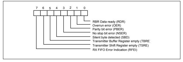
Bit 7: RFEI. In 16450 mode, this bit is always set to a logic 0. In 16550 mode, this bit is set to a logic 1 when there is at least one parity bit error, no stop bit error or silent byte detected in the FIFO. In 16550 mode, this bit is cleared by reading from the USR if there are no remaining errors left in the FIFO.
