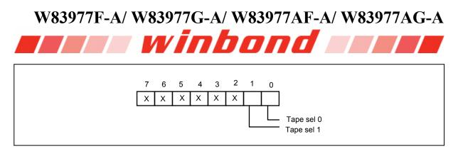
If three mode FDD function is enabled (EN3MODE = 1 in Logical Device 0 CRF0 bit:0), the bit definitions are as follows:
