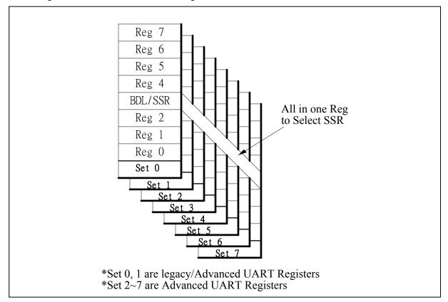
Each of these register sets has a common register, namely *Sets Select Register* (SSR), in order to switch to another register set. The summary description of these *Sets* is shown in the following.
