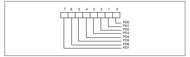
When accesses are made to any EPP data port, the contents of DB0-DB7 are buffered (non-inverting) and output to the ports PD0-PD7 during a write operation. The leading edge of  $\overline{IOW}$  causes an EPP data write cycle to be performed, and the trailing edge of  $\overline{IOW}$  latches the data for the duration of the EPP write cycle.
