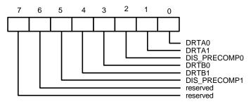
This register controls the data rate selection for FDC. It also controls if precompensation is enabled.
