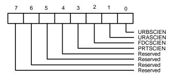
These bits are used to enable the device's IRQ sources onto the SCI logic. The SCI logic output for the IRQs is as follows:
