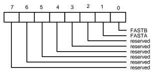
This register is used for the high speed modem application. While the bit is set to logic 1 it can make the baudrate of UART up to 921.2KBPS (the clock source of UART is 14.769MHz) for high speed transmit/receive.
