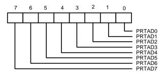
This register is used to select the base address of the parallel port. If EPP is disable, the parallel port can be set from 100H-3FCH on 4-byte boundaries. If EPP is enable, the parallel port can be set from 100H-3F8H on 8-byte boundaries. NCS = 0 and A10 = 0 are required to access the parallel port when in compatible, bi-directional, or EPP modes. A10 is active in ECP mode.
