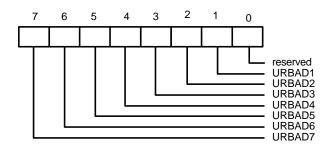
This register is used to select the base address of the UART B from 100H-3F8H on 8-byte boundaries. NCS = 0 and A10 = 0 are required to access the UART B registers. A[2:0] are don't-care conditions.
