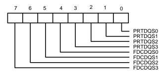
FDCDQS3-FDCDQS0 (Bit 7-bit 4): Allocate DMA resource for FDC. PRTDQS3-PRTDQS0 (Bit 3-bit 0): Allocate DMA resource for PRT.
