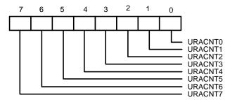
URACNT7 - URACNT0 (Bit 7 - bit 0): UART A idle timer count.
