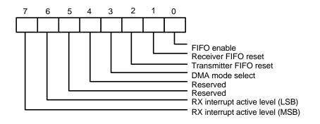
Bit 6, 7: These two bits are used to set the active level for the receiver FIFO interrupt. For example, if the interrupt active level is set as 4 bytes, once there are more than 4 data characters in the receiver FIFO, the interrupt will be activated to notify the CPU to read the data from the FIFO.
