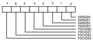
FDCIQS3-FDCIQS0 (Bit 7-bit 4): Allocate interrupt resource for FDC. IQNIQS3-IQNIQS0 (Bit 3-bit 0): Allocate interrupt resource for IRQIN.
