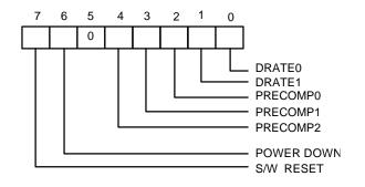
S/W RESET (Bit 7): This bit is the software reset bit.
