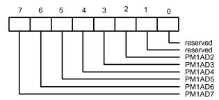
PM1AD7 - PM1AD2 (Bit 7 - bit 2): Base address of the power management register block PM1.
