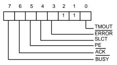
Bit 7: This signal is active during data entry, when the printer is off-line during printing, when the print head is changing position, or during an error state. When this signal is active, the printer is busy and cannot accept data.
