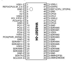
**Note:** Signal names in parenthesis denotes function is selectable through mode pin register strapping.
