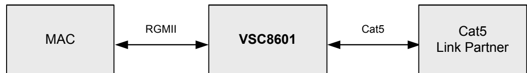
Figure 3. RGMII to Cat5 Block Diagram
