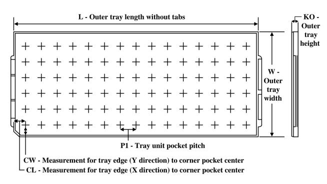
Chamfer on Tray corner indicates Pin 1 orientation of packed units.
