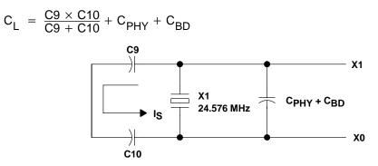
Figure 8–4. Load Capacitance for the TSB43AB23 PHY
