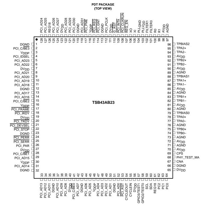
Figure 2–1. PDT Package Terminal Assignments
