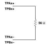
Figure 9–1. Test Load Diagram
