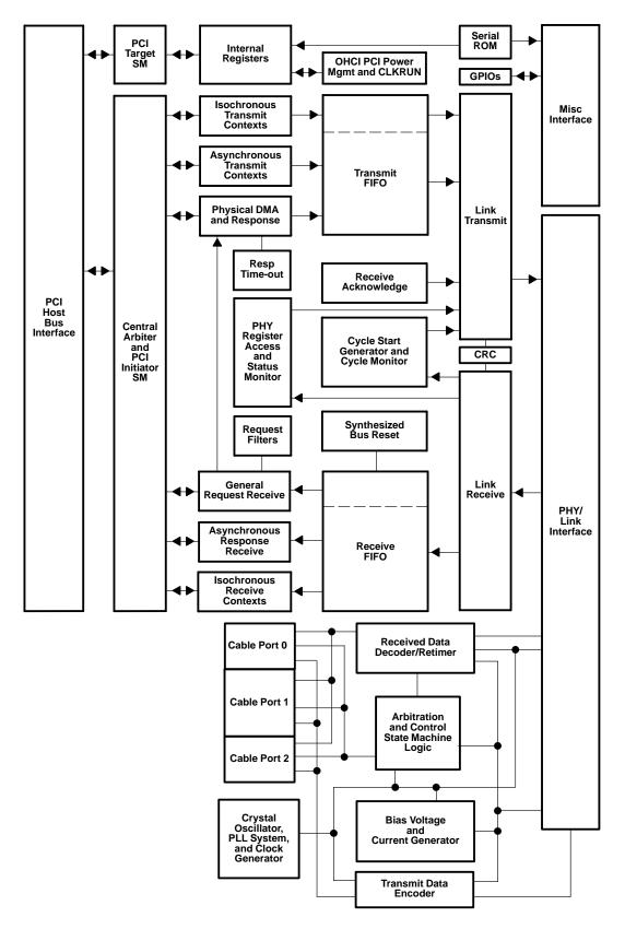
Figure 3–1. TSB43AB23 Block Diagram
