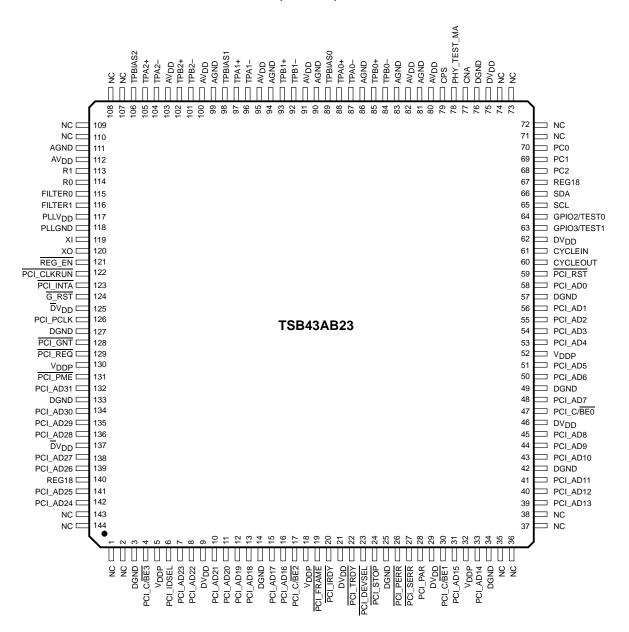
Figure 2–2. PGE Package Terminal Assignments
