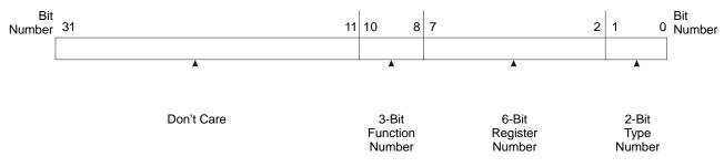
PCI-649 only responds to Type 0 configuration cycles. Type 1 cycles, which pass a configuration request on to another PCI bus, are ignored.
