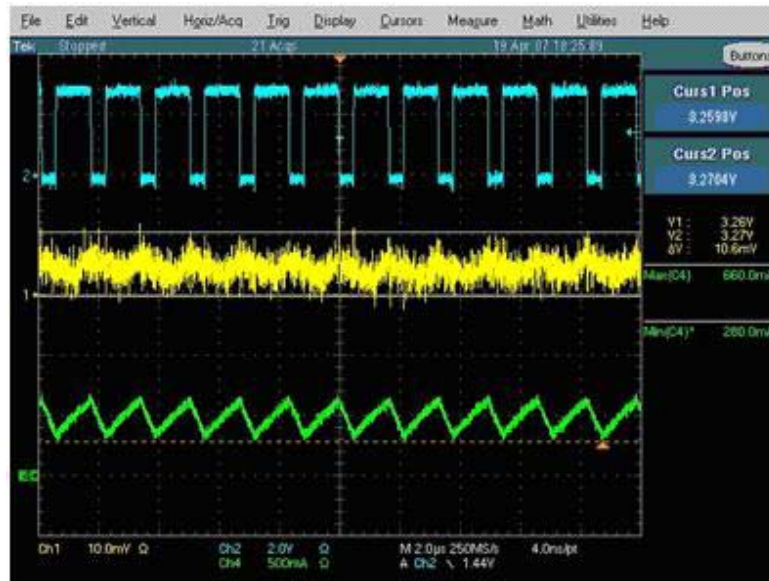
Figure 9. Ceramic 22 \mu F 1210(X5R) (Good)
