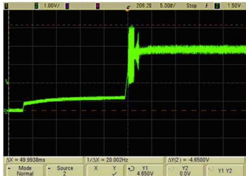
Figure 8. Input Voltage Overshoot >4V (Bad)
