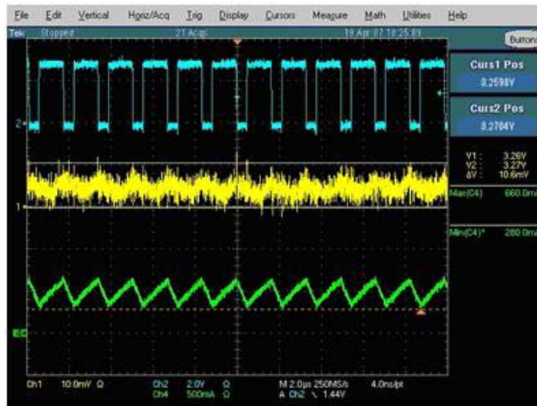
Figure 9. Ceramic 22µF 1210(X5R) (Good)
