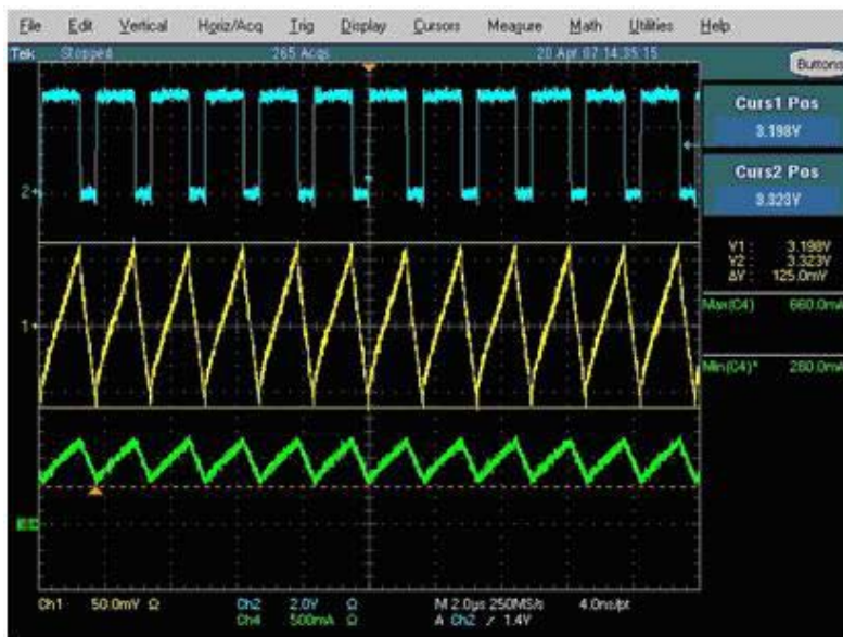
Figure 11. Electrolytic 100 \mu F (Ripple Too High)
