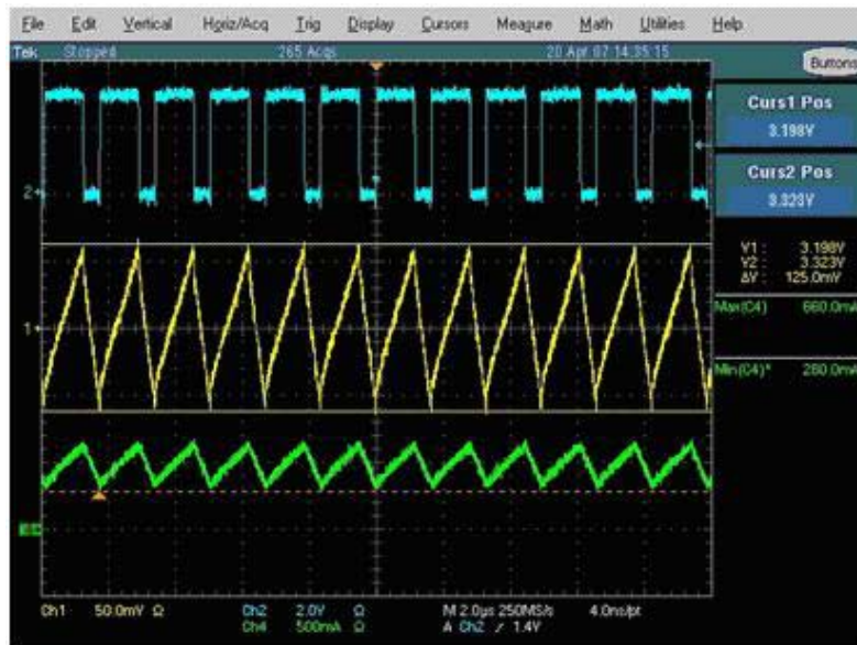
Figure 11. Electrolytic 100 \mu F (Ripple Too High)
