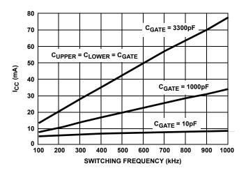
FIGURE 2. BIAS SUPPLY CURRENT vs FREQUENCY
