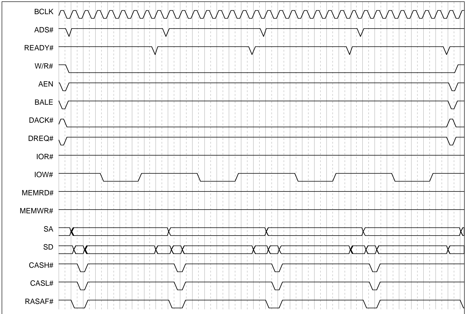
Figure A7-C: R380EX DMA DRAM Read to ISA I/O Write Timing Waveforms
