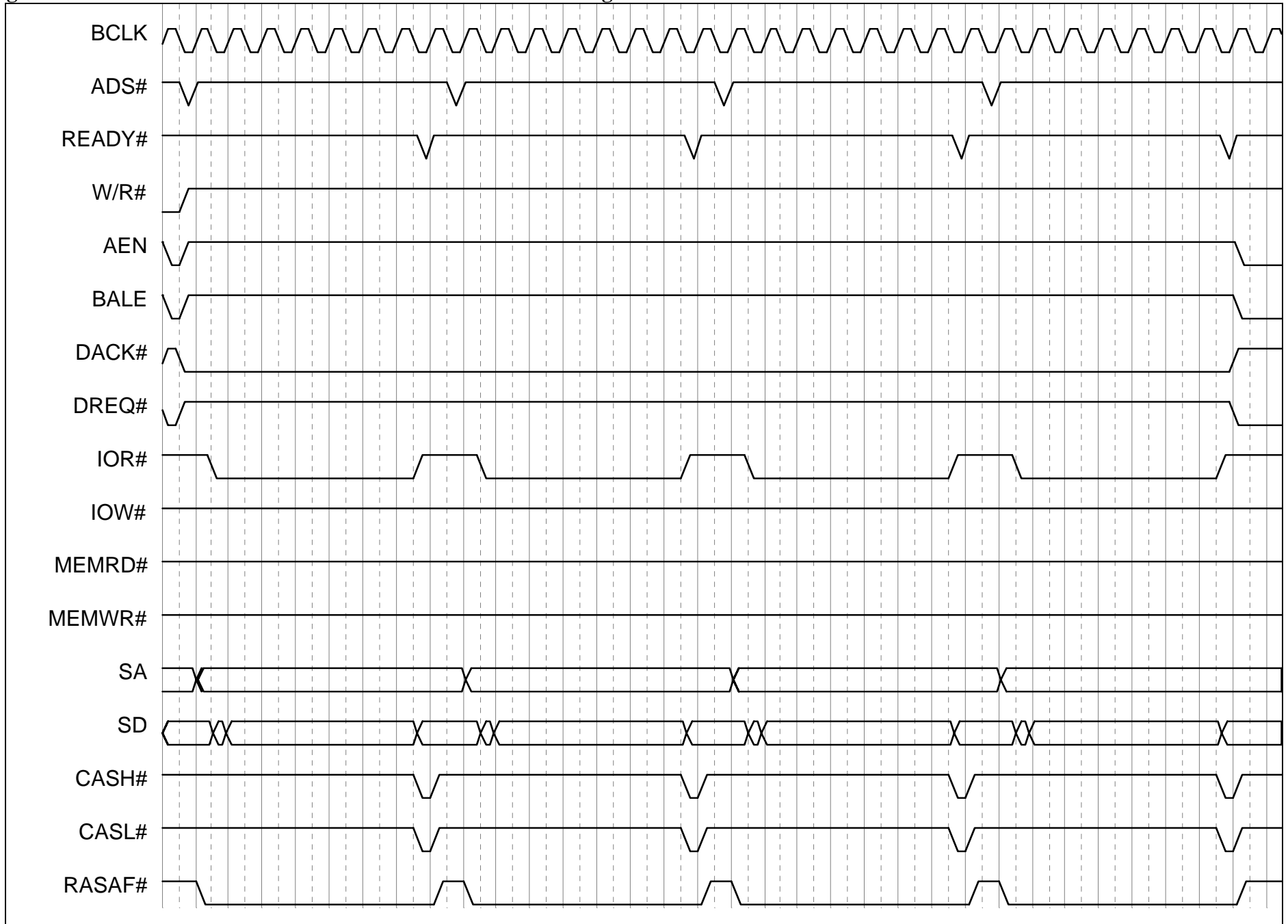
Figure A7-D: R380EX DMA ISA I/O Read to DRAM Write Timing Waveforms
