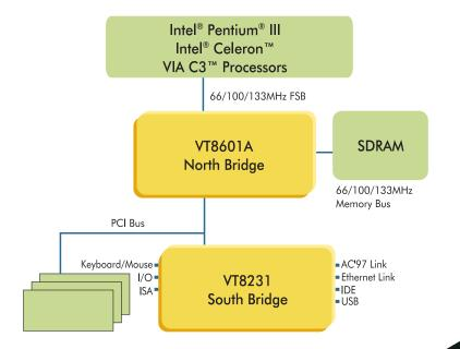
features as a 133MHz Front Side Bus and 133MHz SDRAM support to deliver unrivaled flexibility and performance in an affordable yet highly-integrated chipset. With its flexible 66/100/133MHz FSB settings, the VIA Apollo PLE133 is designed to optimize the performance of a full range of Intel® Pentium® III, Intel® Celeron™, and VIA C3™ processors. Its support for PC133 SDRAM ensures ample memory bandwidth for the most demanding software and Internet
