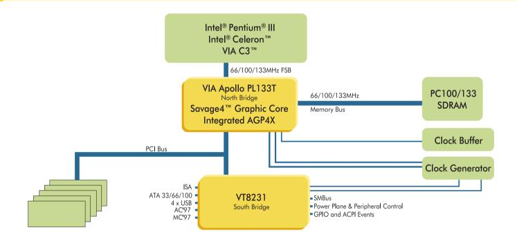
The VIA Apollo PL133T offers exceptional graphics performance provided by an advanced S3 Savage4™ 3D/2D graphics core and integrated AGP4X. Combined with PC133 SDRAM and ATA-100 technologies it redefines the integrated chipset standard for the mainstream and value markets. The VIA Apollo PL133T also offers complete flexibility with adjustable 66/100/133MHz Front Side Bus, PC66/100/133MHz SDRAM and VCM support.
