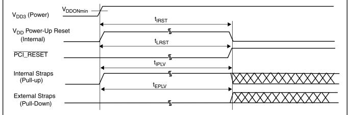
Figure 47. Internal  $V_{DD}$  Power-Up Reset
