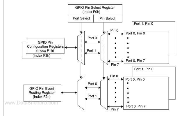
Figure 10. Organization of GPIO Pin Registers GPCFG1-2, GPEVR and GPMODE
