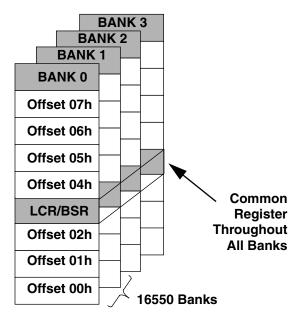
Figure 38. Register Bank Architecture
