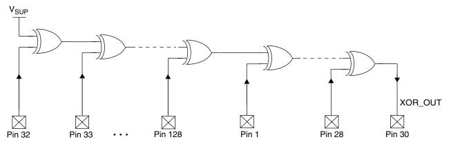
Figure 3. XOR Tree (Simplified Diagram)
