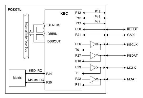
Figure 41. Keyboard and Mouse Interfaces
