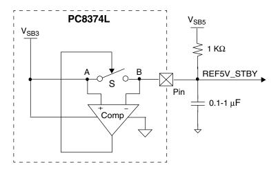
Figure 21. REF5\_STBY Generation (Simplified Diagram)
