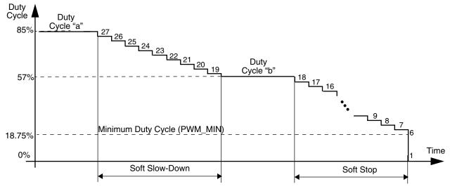
Figure 34. Soft Slow-Down and Soft Stop Example
