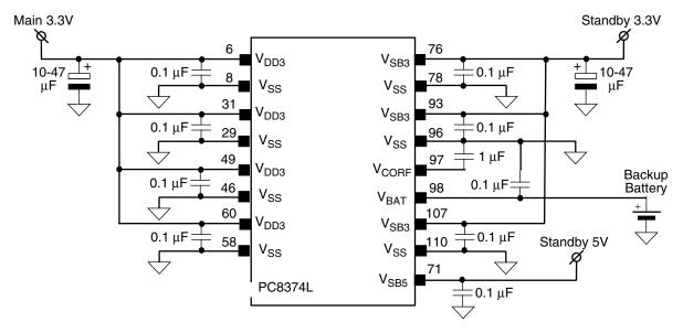
Figure 2. Decoupling Capacitors Connection
