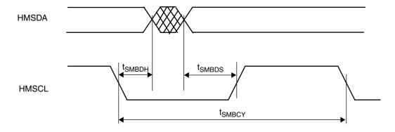
Figure 59. SMBus Data Bit Timing
