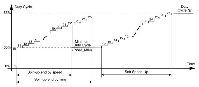
Figure 33. Soft Spin-Up and Soft Speed-Up Example
