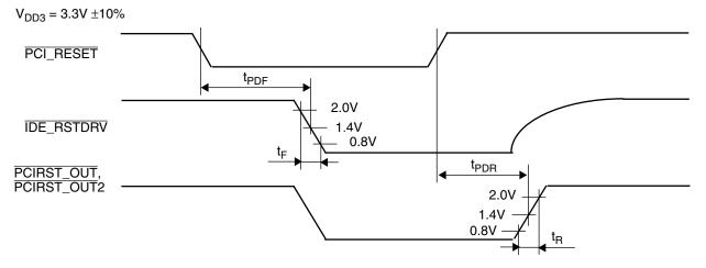
Figure 54. Reset Outputs
