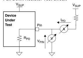
Figure 42. Internal Resistor Test Conditions,  $T_A = 0$ °C to 70°C,  $V_{SUP} = 3.3V$
