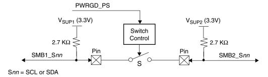
Figure 29. SMBus Isolation (Simplified Diagram)
