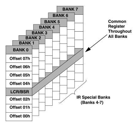
Figure 39. SP2 Register Bank Architecture
