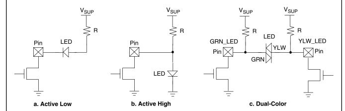
Figure 14. LED Connection Configurations
