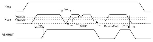
Figure 23. RSMRST at V<sub>SB5</sub> and V<sub>SB3</sub> Switching
