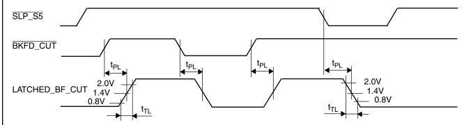
Figure 55. BKFD\_CUT and LATCHED\_BF\_CUT (AC Characteristics)
