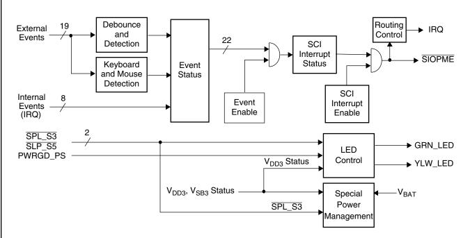
Figure 11. SWC Block Diagram
