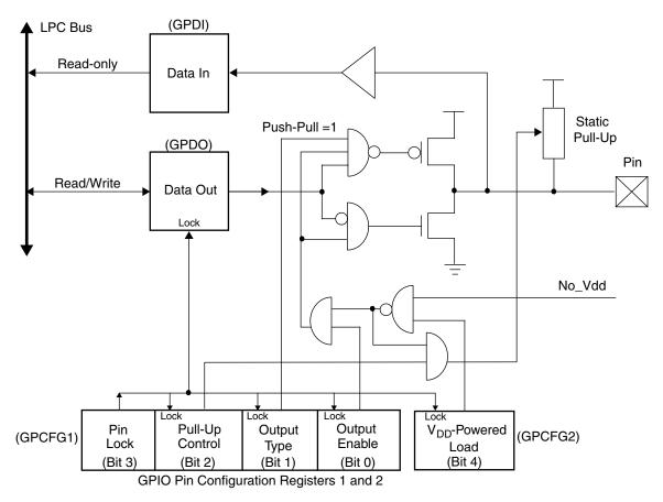
Figure 16. GPIO Basic Functionality
