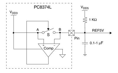
Figure 19. REF5 Generation (Simplified Diagram)
