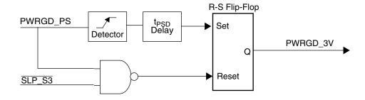
Figure 24. PWRGD\_3V Generation (Simplified Diagram)
