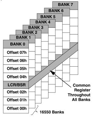
Figure 40. Register Bank Architecture
