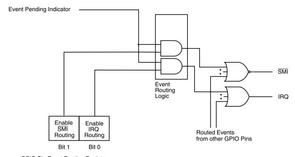
GPIO Pin Event Routing Register
