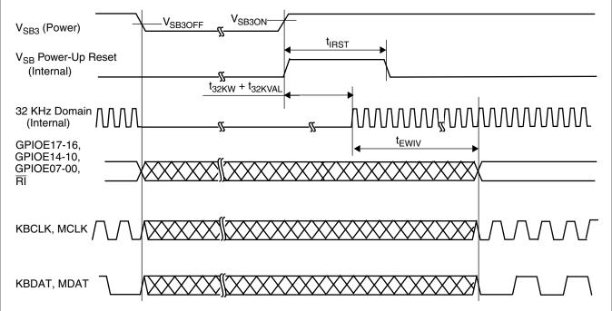
Figure 56. Inputs at V<sub>SB3</sub> Power Switching
