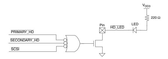
Figure 27. HD\_LED Generation (Simplified Diagram)
