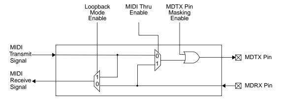
Figure 34. MIDI Signals Routing Control Logic
