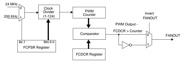
Figure 14. PWM Generator (FANOUT)
