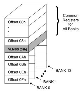
Figure 38. Register Bank Architecture
