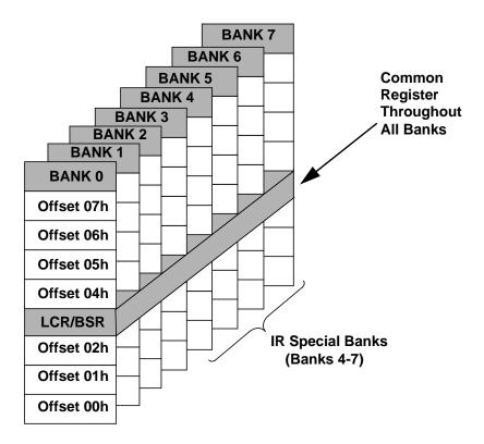
Figure 48. SP2 Register Bank Architecture
