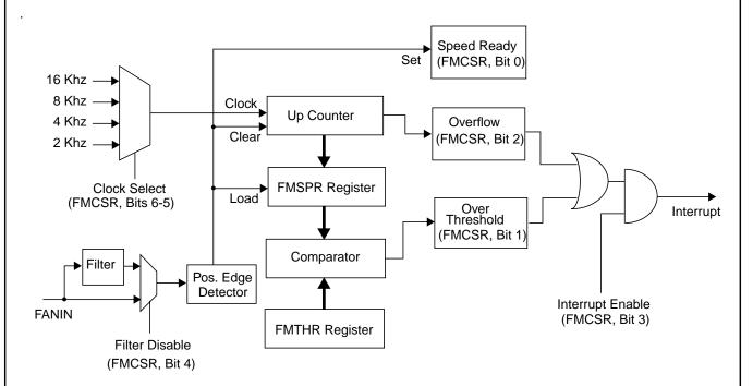
Figure 16. Fan Speed Monitor
