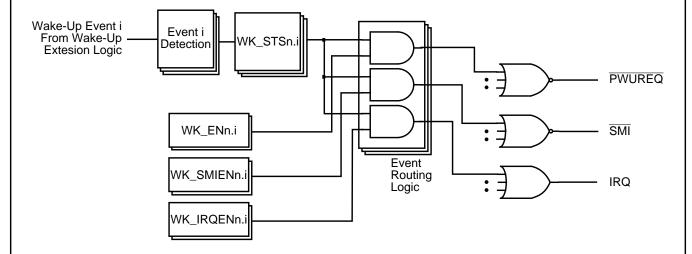
Figure 8. Wake-Up Events Routing Scheme
