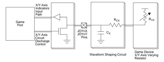
Figure 28. Game Device Axis Position Indication Mechanism
