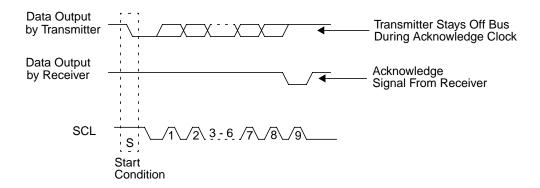
Figure 25. ACCESS.bus Acknowledge Cycle
