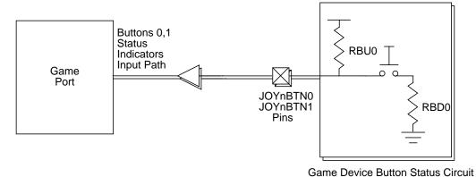
Figure 30. Game Device Button Status Indication Mechanism
