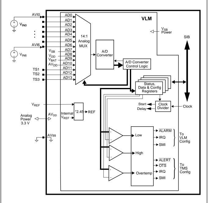
Figure 35. VLM Functional Diagram
