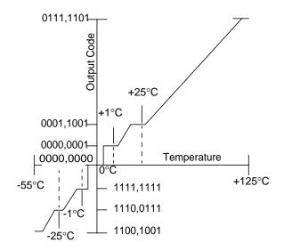
Figure 44. Temperature-to-Digital Transfer Function (Non-linear scale for clarity)
