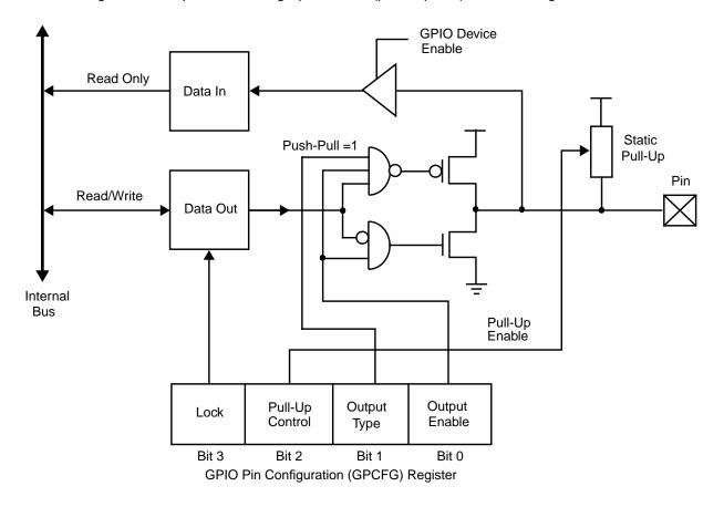
Figure 18. GPIO Basic Functionality
