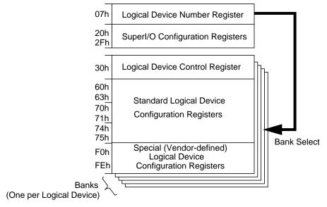
Figure 2. Structure of the Standard Configuration Register File
