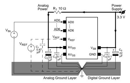
Figure 37. Analog Power Supply
