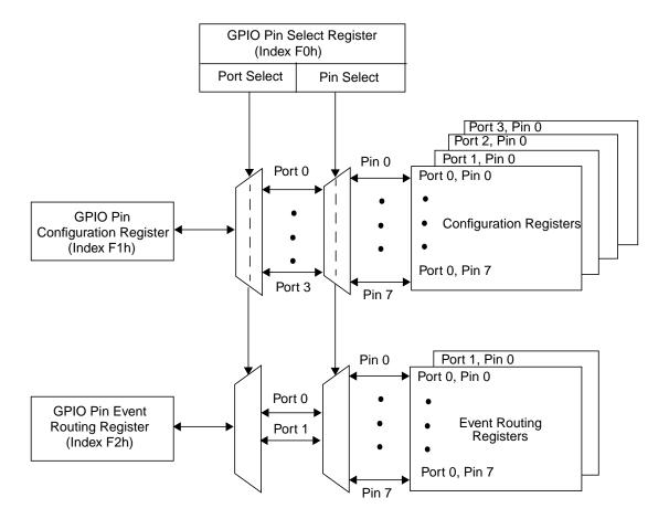
Figure 6. Organization of GPIO Pin Registers
