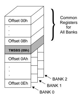
Figure 42. Register Bank Architecture
