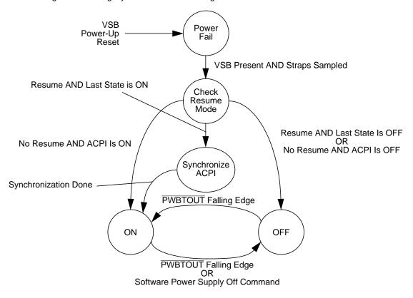
Figure 4. Legacy Power Supply Control State Diagram
