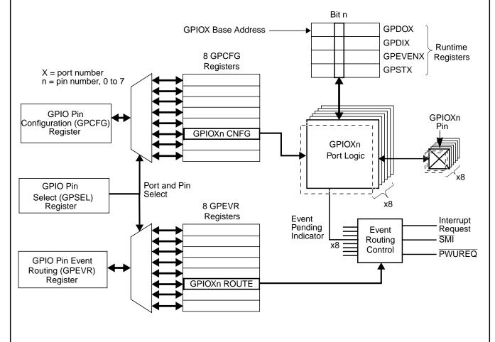
Figure 17. GPIO Port Architecture
