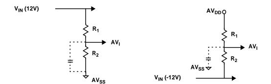
Figure 40. Measurement of Positive and Negative Voltages
