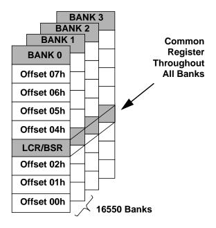
Figure 47. UART Mode Register Bank Architecture
