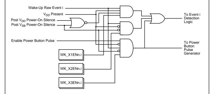
Figure 9. Wake-Up Mode Control (Extension) Mechanism
