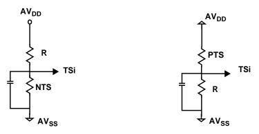
Figure 36. Measuring Temperature using Thermistors
