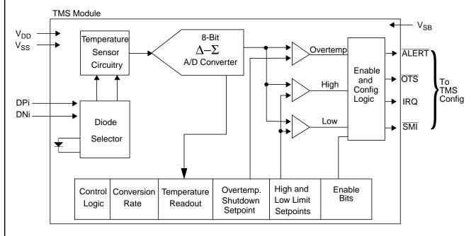
Figure 41. TMS Simplified Block Diagram
