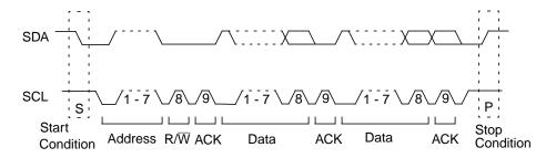
Figure 26. A Complete ACCESS.bus Data Transaction
