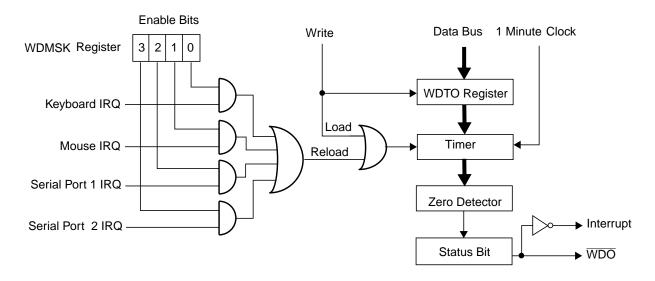
Figure 21. WATCHDOG Timer Functional Diagram
