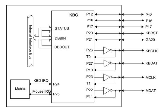
Figure 5. Keyboard and Mouse Interfaces
