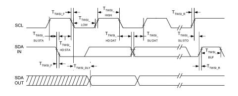
Figure 80: Two-Wire Serial Interface Timing
