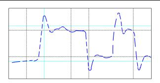
Figure 39: Signal Reflections, using the 50 ohm Setting, 60 ohm line
