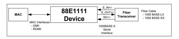
There are two modes of fiber operation. Table 31 shows the mode to select digital interfaces connecting to fiber media.
