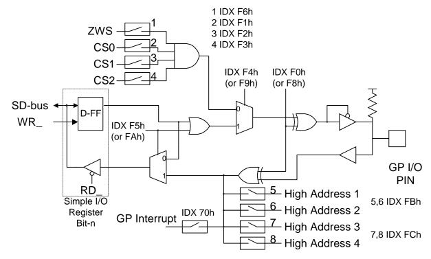
Note: All GPIO pins are internally pulled up 50 K $\Omega$  except GPIO10 (pin 19).
