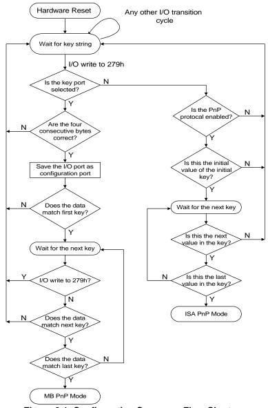
Figure 6-1. Configuration Sequence Flow Chart
