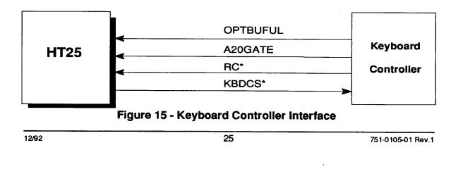
OPTBUFUL furnishes the interrupt request number one to the HT25's interrupt controller. This signal is normally used to indicate that there is keyboard information in the keyboard controller for the system to read.
