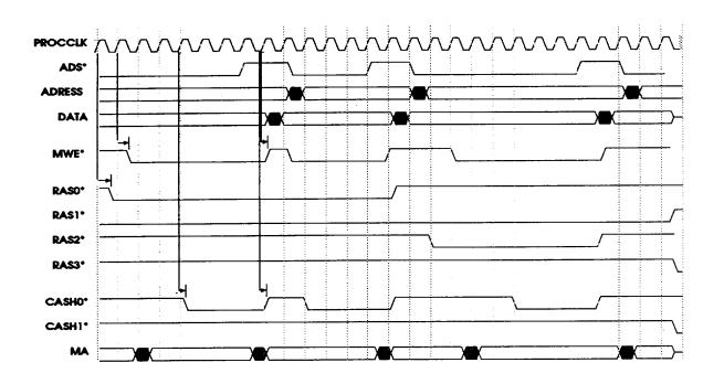
Figure 10d - Extended Timing (Write), Page Miss/Hit
