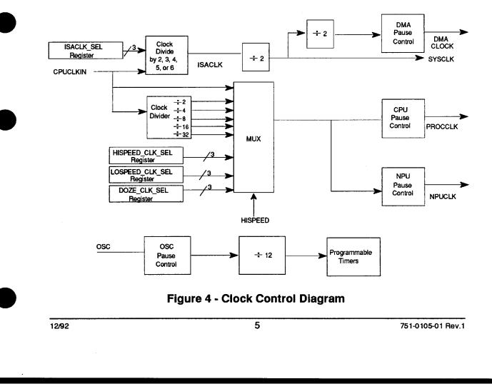
the CPU clock remains active to allow for servicing the interrupt is controlled by the Interrupt Control Register if bit 7 is a 1. This allows housekeeping interrupts (SMI is not set to occur) to be handled and quickly stop the clock again. If the SMI enable bit is on for an interrupt, the SMM code will usually clear the CPU stop clock bit to keep the clock running when that interrupt occurs. If bit 7 is set to 0 the CPU clock will restart only for interrupts which have their SMI enable bit set.
