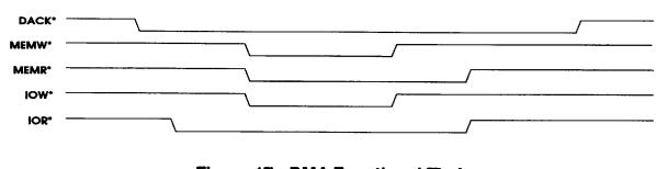
Figure 17 - DMA Functional Timing
