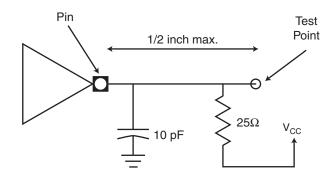
Figure 7. TVAL (min) Test Load
