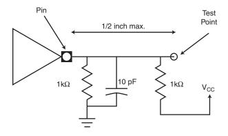
Figure 8. TVAL Test Load (PCI 5 V Signaling Environment)
