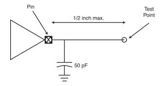
NOTE: Note: 50 pF load used for maximum times. Minimum times are specified with 0 pF load.
