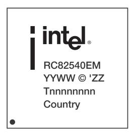
Figure 10. 82540EM Device Identification Markings
