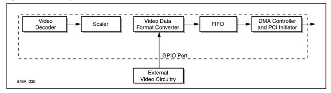
The GPCLK signal is used to input an external clock signal. The video data and related signals are accepted over the GPIO pins, defined in Table 3-2.
