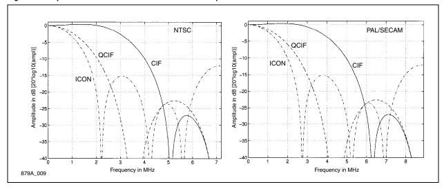
Figure 2-6. Combined Luma Notch, 2x Oversampling and Optional Low-Pass Filter Response (NTSC)
