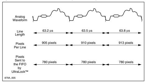
UltraLock can be used to extract any programmable number of pixels from the original video stream as long as the sum of the nominal pixel line length (910 for NTSC and 1,135 for PAL/SECAM) and the worst case line length validation from nominal in the active region is greater than or equal to the required number of output pixels per line; i.e.,
