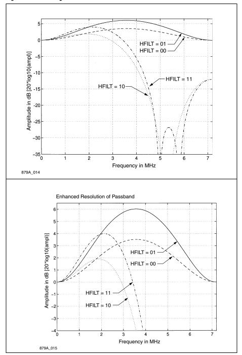
Figure 2-11. Luma Peaking Filters with 2x Oversampling Filter and Luma Notch (1 of 2)
