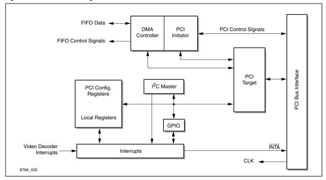
Figure 3-5. PCI Audio Block Diagram
