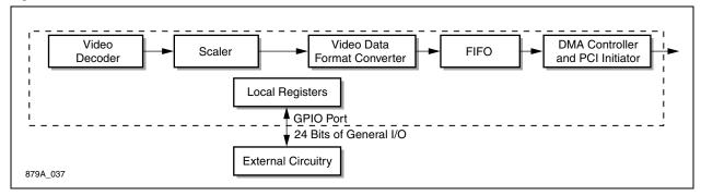
Data is written to and read from the GPIO pins through the GPDATA signal. When configured to output signals through the GPIO, information is written to a GPDATA holding register, which is output to the pin. When configured to input data from the GPIO, buffered data is read directly from the pin. Illustrated in Figure 3-6.
