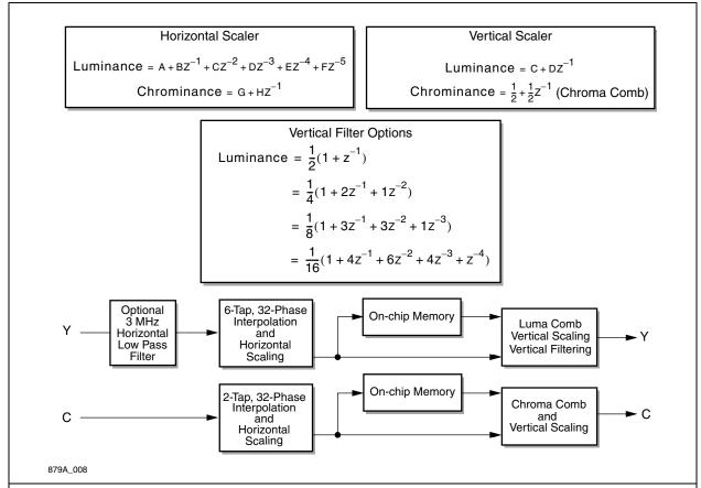
**NOTE(S):** Z<sup>-1</sup> refers to a pixel delay in the horizontal direction, and a line delay in the vertical direction. The coefficients are determined by UltraLock and the scaling algorithm.
