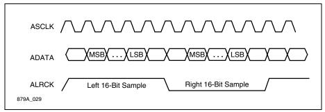
There can be any number of ASCLKs  $\geq$  16 (usually 16–32 between ALRCK edges. Thus there may be extra ASCLKs versus collected data bits. There is no requirement for ASCLK (or ALRCK or ADATA)) to be continuous. A specified edge of ASCLK is used to sample the other two signals. Each 16-bit sample is sampled a specified number of ASCLK edges from the edge of ALRCK, which serves as a word sync.
