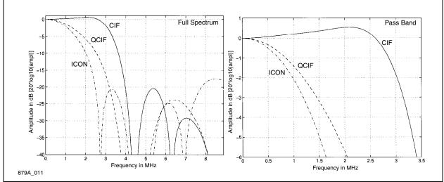
Figure 2-8. Combined Luma Notch and 2x Oversampling Filter Response
