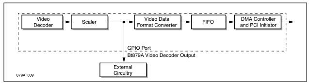
When running the GPIO port in SPI Output mode, the GPCLK is configured to output CLKx1 ( $4 \times Fsc$ ). CCIR601 is followed when the RANGE bit is set to 0. The GPIO pins are mapped as described in Table 3-3.
