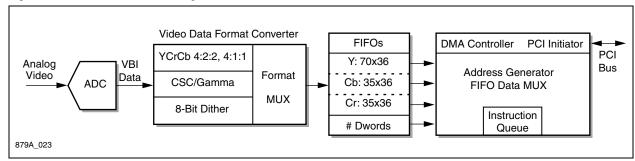
In the VBI frame output mode, VBI data capture occurs in the active video region and includes all the horizontal blank/sync information in the data stream. This feature can be used to provide a high quality still-capture of video. The data is vertically bound beginning at the first line during VACTIVE and ending after a fixed number of packets. The data stream is packetized into a series of 256-DWORD blocks.
