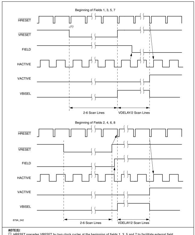
(1) HRESET precedes VRESET by two clock cycles at the beginning of fields 1, 3, 5 and 7 to facilitate external field generation.
