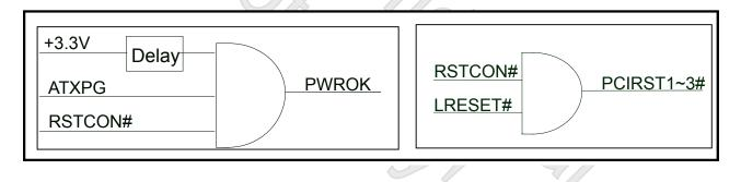
So far as the PWROK issue is as the figure above. PWROK is delayed 400ms (default) as VCC arrives 2.8V, and the delay timing can be programmed by register. (100ms ~ 400ms)
