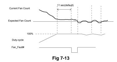
(2). After the period of detecting fan full speed, when PWM\_Duty > Min. Duty, and fan count still in 0xFFF.
