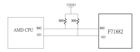
In Intel SST and PECI interfaces, the F71882 can connect to CPU/SST directly. The F71882 can read the temperature data from CPU, than the fan control machine of F71882 can implement the Fan to cool down CPU temperature. As same as PECI, chipset can get information from F71882 including CPU temperature, system temperature (F71882 provides D+/D- for system temperature sensing), fan speed status by SST. The application circuit is as below. More detail please refer the register description.
