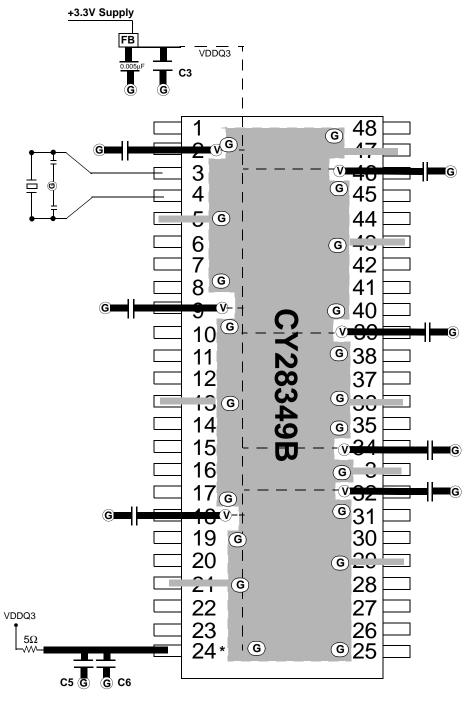
$\bigcirc$  = VIA to GND plane layer  $\bigcirc$  =VIA to respective supply plane layer
