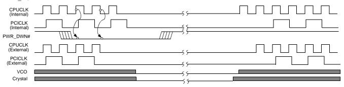
Shaded section on the VCO and Crystal waveforms indicates that the VCO and crystal oscillator are active, and there is a valid clock.
