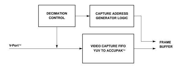
Figure 2-9. V-Port™ Functional Block Diagram
