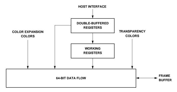
Figure 2-8. BitBLT Engine
