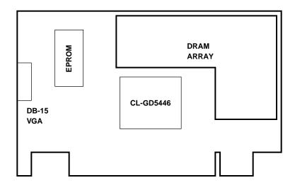
Figure B1-1. PCI Bus Adapter Card Layout
