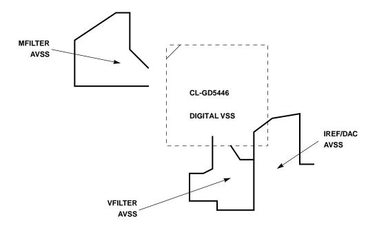
Figure B1-3. Ground Plane Layout
