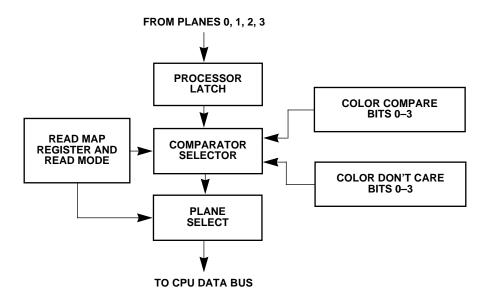
Figure 2-4. Graphics Controller Read Operation
