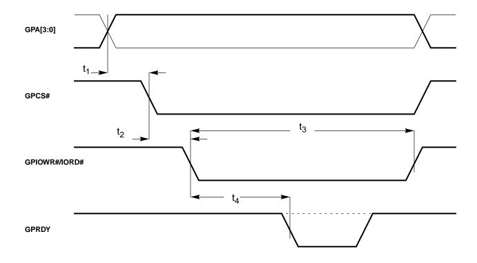
Figure B11-1. GPIO Timing: RDY Termination
