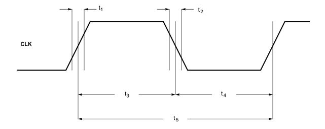
Figure 11-1. CLK Timing (PCI Bus)
