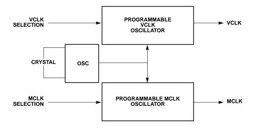
Figure 2-6. Programmable Dual-Frequency Synthesizer Functional Diagram
