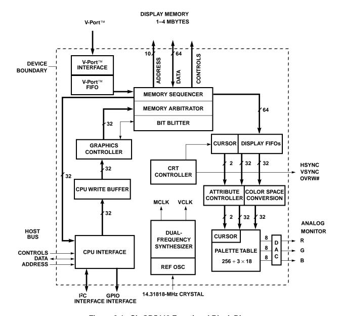
Figure 2-1. CL-GD5446 Functional Block Diagram
