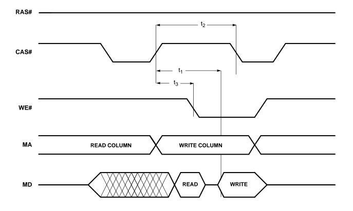
Figure 11-15. Display Memory Bus: BitBLT Read/Write Cycle
