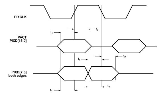
Figure 11-18. V-Port™: PIXCLK Timing
