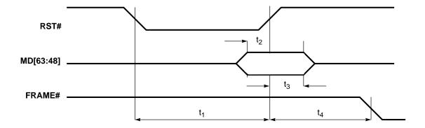
Figure 11-20. Reset Timing
