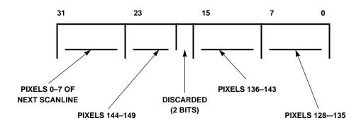
Figure 9-19. Text Expansion Example
