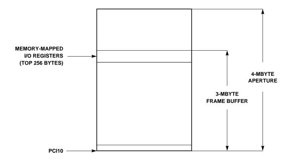
Figure 9-17. Memory-Mapped I/O in Linear Aperture
