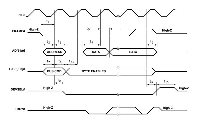
Figure 11-2. FRAME#, DEVSEL#, AD[31:0], and C/BE[3:0]# (PCI Bus)
