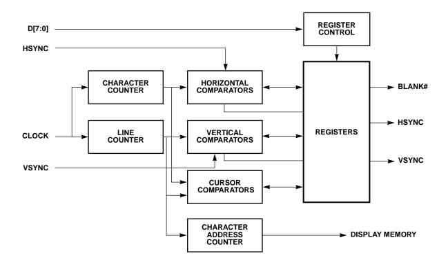
Figure 2-2. CRT Controller Functional Block Diagram
