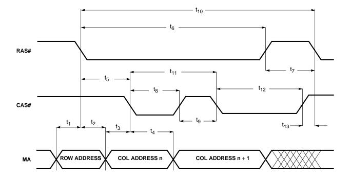
Figure 11-13. Display Memory Bus: Common Parameters (EDO Timing)
