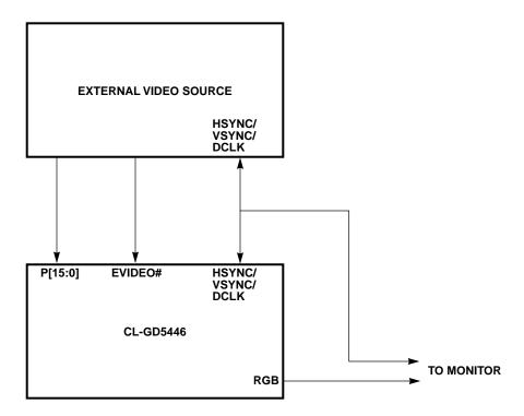
Figure 9-23. SWITCH with EVIDEO#
