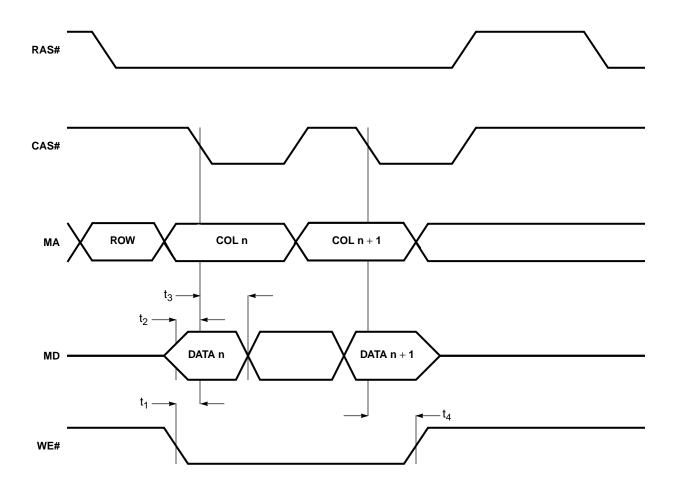
Figure 11-12. Display Memory Bus: Write Cycles
