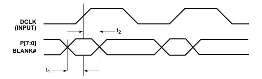
Figure 11-16. P-Bus as Inputs: 8-Bit Mode (External DCLK)
