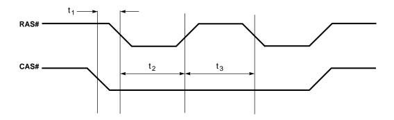
Figure 11-9. Display Memory Bus: CAS#-before-RAS# Refresh Timing
