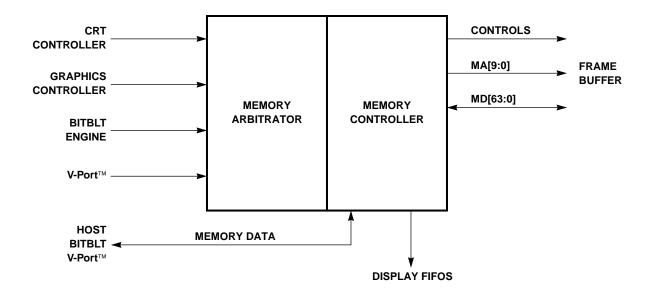
Figure 2-1. Sequencer Functional Block Diagram
