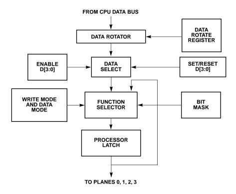
Figure 2-3. Graphics Controller Write Operation
