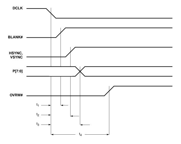
Figure 11-17. Feature Bus Timing: 8-bit Mode, Output (Internal DCLK)
