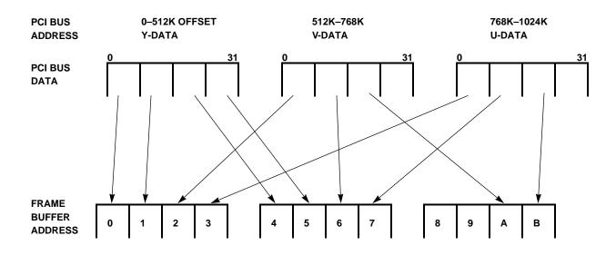
Figure 9-1. Frame Buffer Video Aperture
