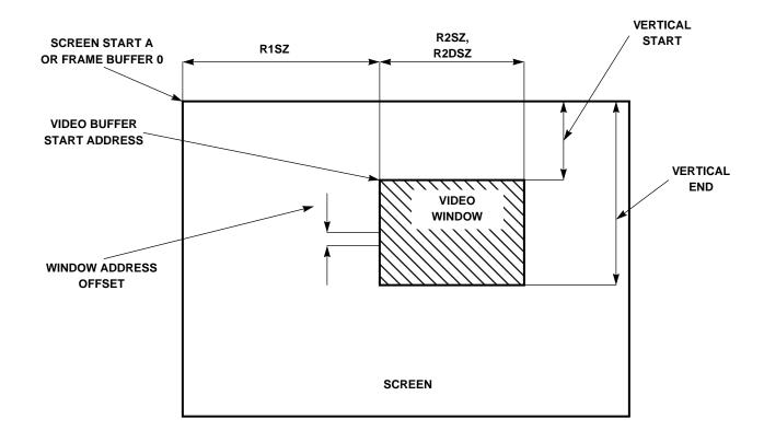
Figure 9-21. Positioning of the Video Window
