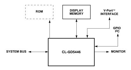
Figure 2-10. Computer Display Subsystem Architecture
