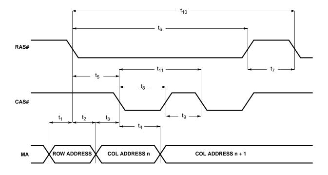
Figure 11-10. Display Memory Bus: Common Parameters (No EDO)
