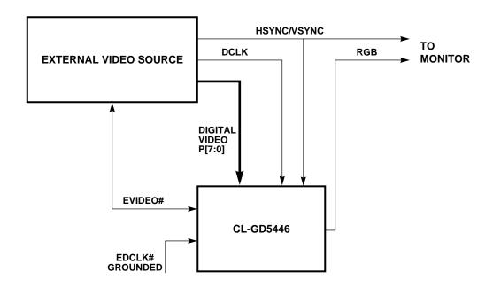
Figure B9-1. Video Overlay Connections
