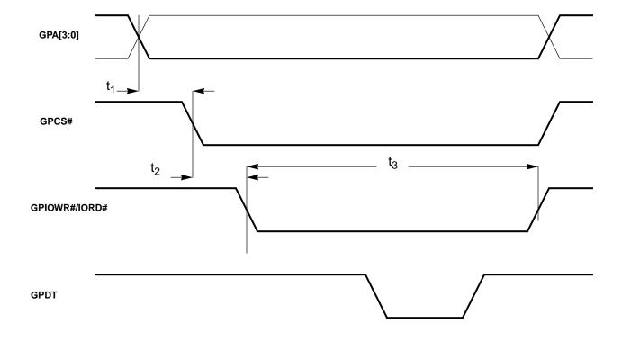
Figure B11-2. GPIO Timing: GPDT Termination
