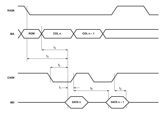
Figure 11-11. Display Memory Bus: Read Cycles
