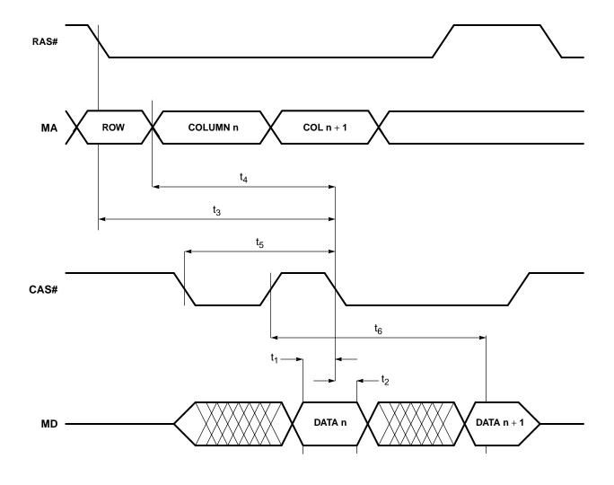
Figure 11-14. Display Memory Bus: Read Cycles (EDO Timing)
