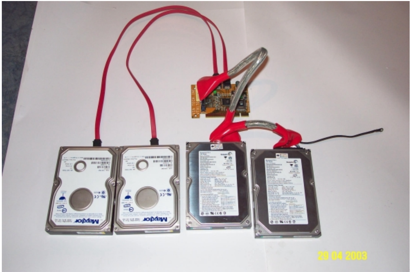
SATA Cabling (left) vs PATA Cabling (right)
