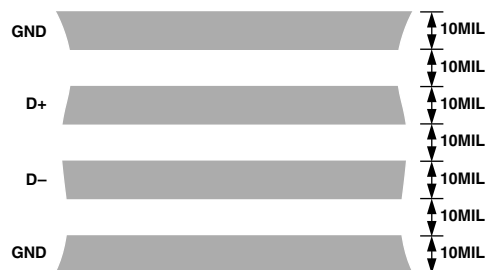
Figure 12. Arrangement of Signal Tracks
