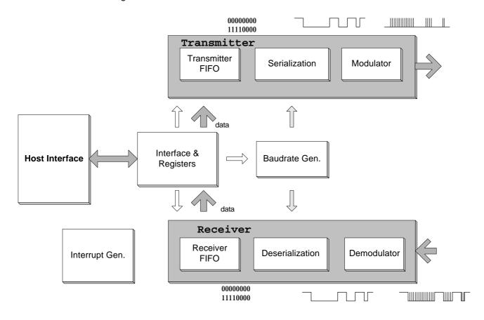
Figure 10-7. CIR Block Diagram
