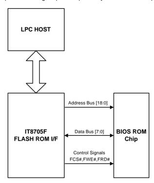
Figure 10-8. FLASH ROM Interface Diagram
