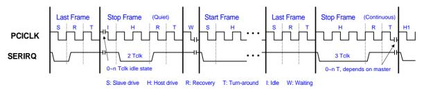
Figure 10-2. Stop Frame Timing
