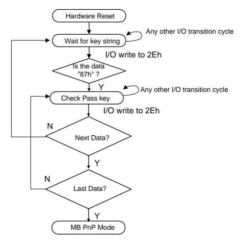
There are three steps to completing the Motherboard mode of configuration. Step one is to enter the MB PnP mode. Step two is modifying the data of configuration registers. Step three is exiting the MB PnP mode. These three steps are explained below. Please note that step three must be followed or an undefined state will occur.
