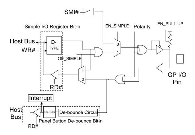
Figure 10-1. General Logic of GPIO Function
