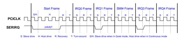
Figure 10-1. Start Frame Timing
