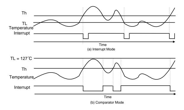
Figure 10-1. Temperature Interrupt Response Diagram
