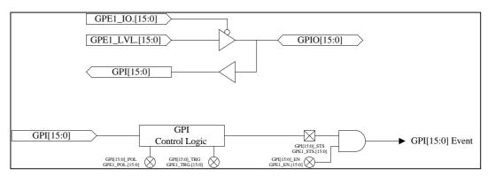
Figure 21.2-3 Hardware Model for Generic Feature 1 (GPE1)
