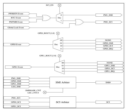
Figure 21.3-1 Interrupt Model for ACPI
