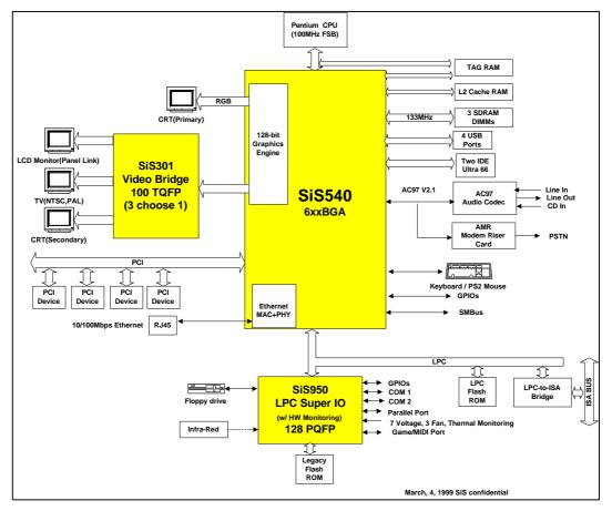
Figure 1-1 SiS540 System Block Diagram
