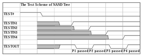
Figure 6.8-2 The Test Scheme of NAND Tree
