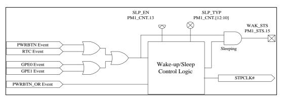
Figure 21.6-1 Hardware Model for PME#
