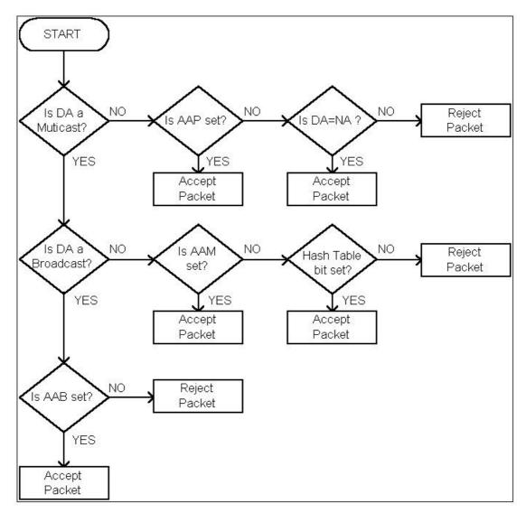
Figure 13.3-1 Receive Filter Algorithm
