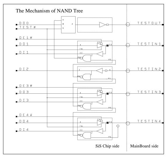
Figure 6.8-1 The Mechanism of NAND Tree
