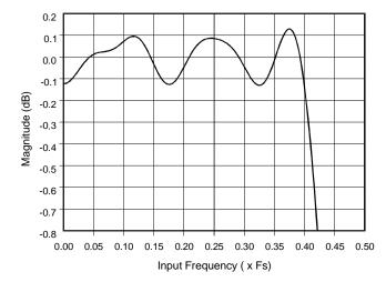
Figure 33. ADC Passband Ripple
