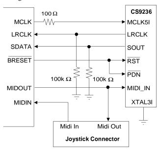
Figure 11. CS9236 Wavetable Serial Port Interface
