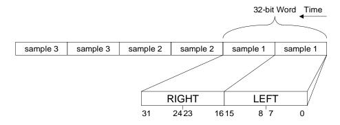
Figure 15. 16-bit Stereo, Signed Little Endian Audio Data
