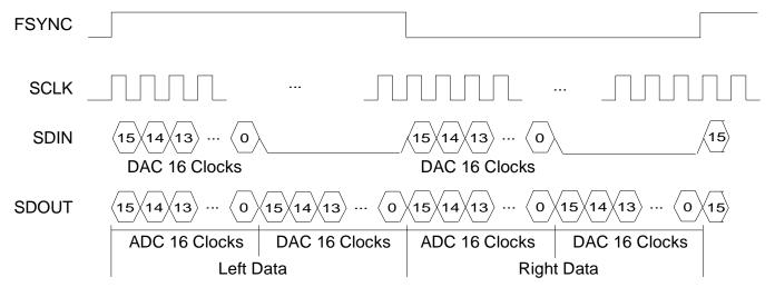
**Figure 10. ADC/DAC Mode (SF1,0 = 11)**
