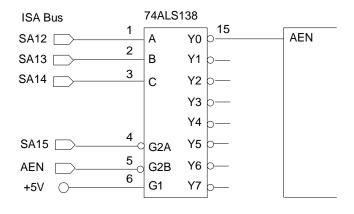
Figure 2. 16-bit Decode Circuit
