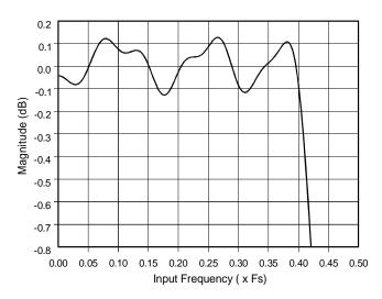
Figure 36. DAC Passband Ripple
