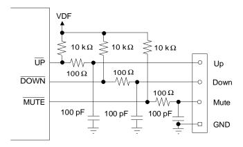
Figure 22. Volume Control Circuit
