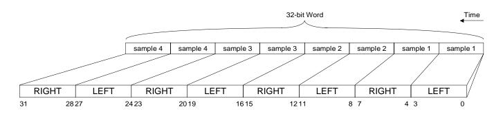
Figure 17. 4-bit Stereo, ADPCM Audio Data
