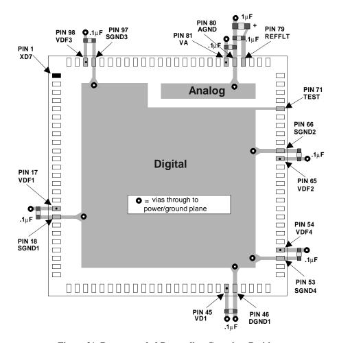
Figure 31. Recommended Decoupling Capacitor Positions
