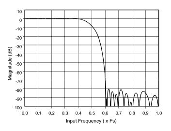
Figure 32. ADC Filter Response
