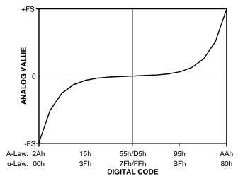
Figure 21. Companded Transfer Functions
