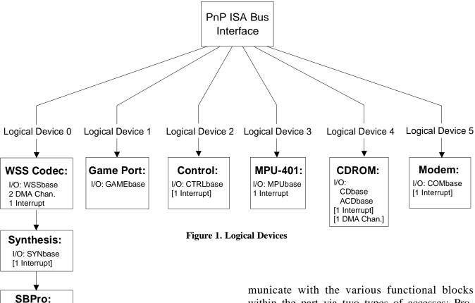
Logical Device 5 supports a modem connected to the peripheral port. This interface, on the external peripheral port, supports modems with 2 to 256 I/O locations (only SA2-SA0 are buffered through the part) and supports a base address and an interrupt. Although this logical device is listed as a modem, any external device that fits within the resources listed above may be substituted.
