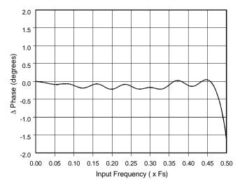
Figure 38. Deviation from Linear Phase
