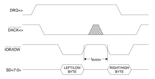
8-Bit Stereo or 16-Bit Mono DMA Cycle
