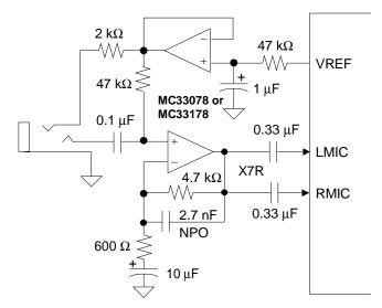
Figure 26. Left or Mono Microphone Input
