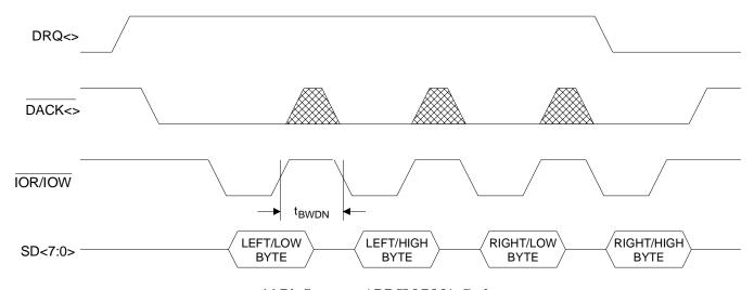
16-Bit Stereo or ADPCM DMA Cycle
