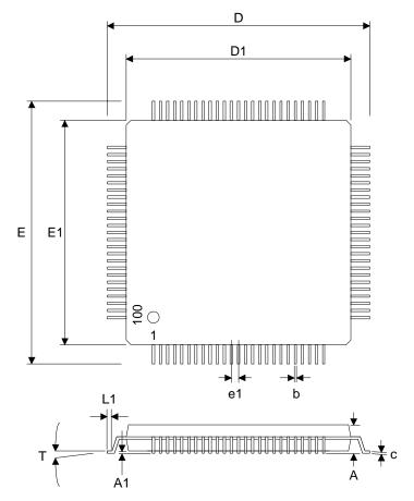
100-pin TQFP - Package Code 'Q'
