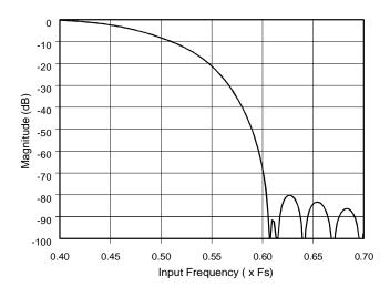
Figure 34. ADC Transition Band
