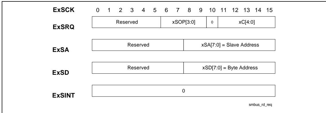
Figure 13. SMBUS SIO Random Read Request Packet Format
