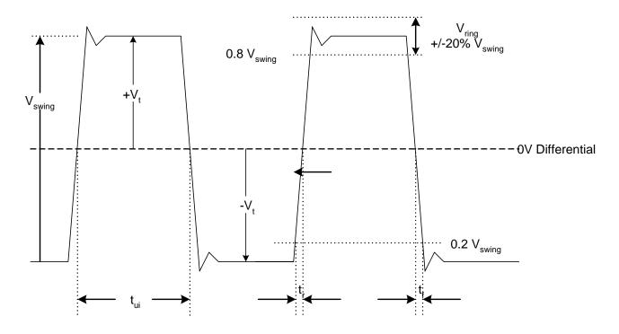
Figure 7: AC Timing for LVDS Outputs
