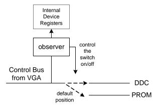
Figure 4: Control Bus Switch
