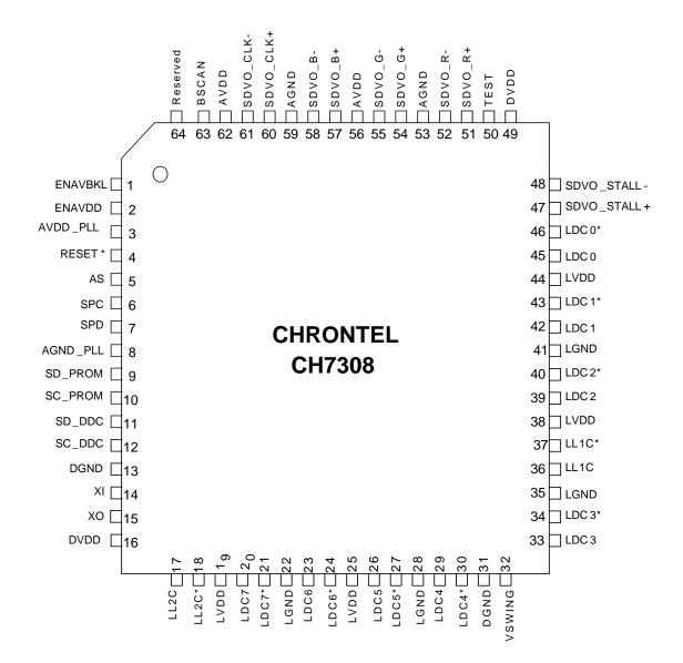
Figure 2: 64 Pin LQFP Pin Out (Top View)
